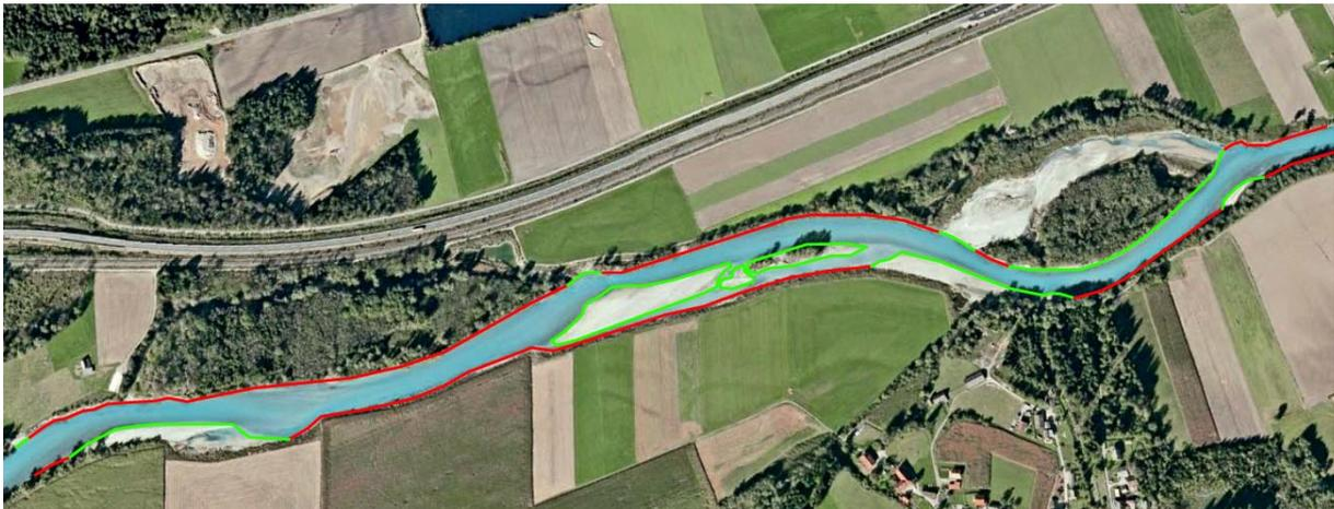
**Figure 7.6 Bank protection constraining the flow at mean discharge in the evaluated reach (restored state in 2008).**
