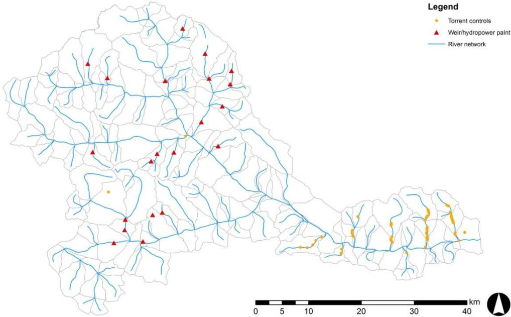
**Figure 7.1 Sediment barriers in the catchment of the investigated reach at the Drau River. Throughput coefficients were defined according to the type of crossing structures.**
