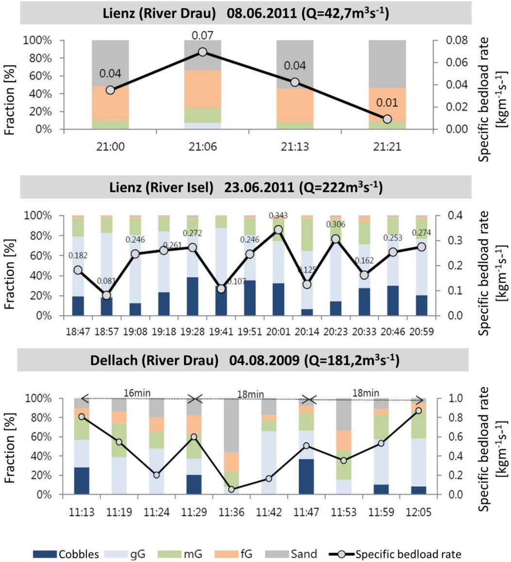
**Figure 4.40** Examples of three continuous bed load measurements with the basket sampler – grain sizes (colored columns) and specific bed load rate (line) (Habersack et al., 2013).
